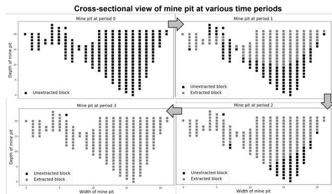
Fig. 1. Block extraction sequence example from year to year following precedence and resource constraints for MineLib’s Newman1 instance [1].
