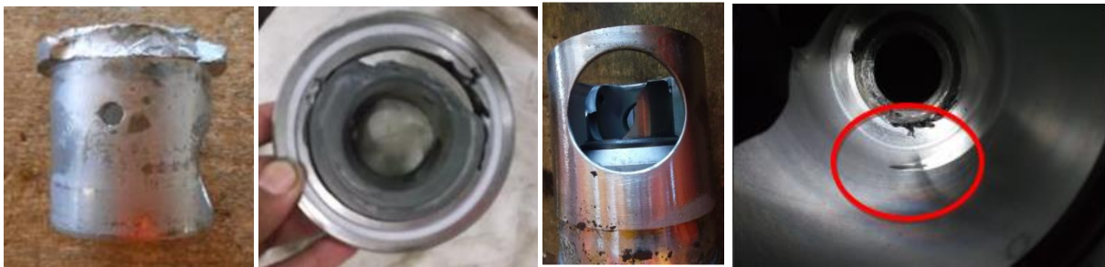
Figure 19 Well 3N choke valve trim damage condition
