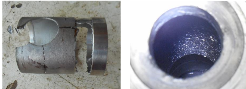
Figure 21 Trim condition of choke valve from well 4J on September 2019
