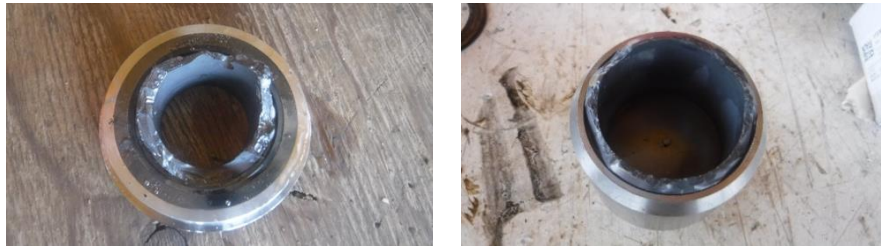
Figure 20 Trim condition of choke valve from well 4J on April 2018
