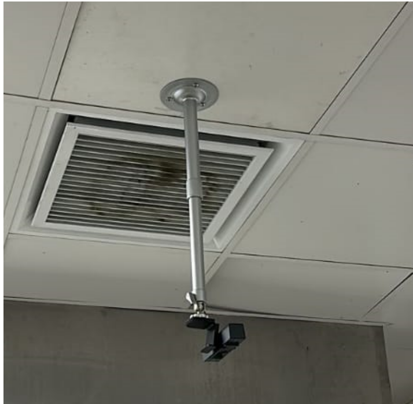
Fig 1: Web camera mounted on ceiling to capture top-down video of conveyor belt-based cutlery washing machine
