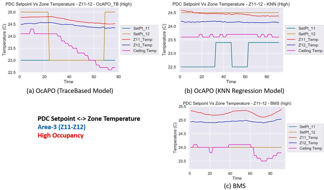
Fig. 13. PDC setPoint by BMS, OcAPO (TraceBased and KNN) Vs ceiling and zone temperature — high occupancy (Area-3).
