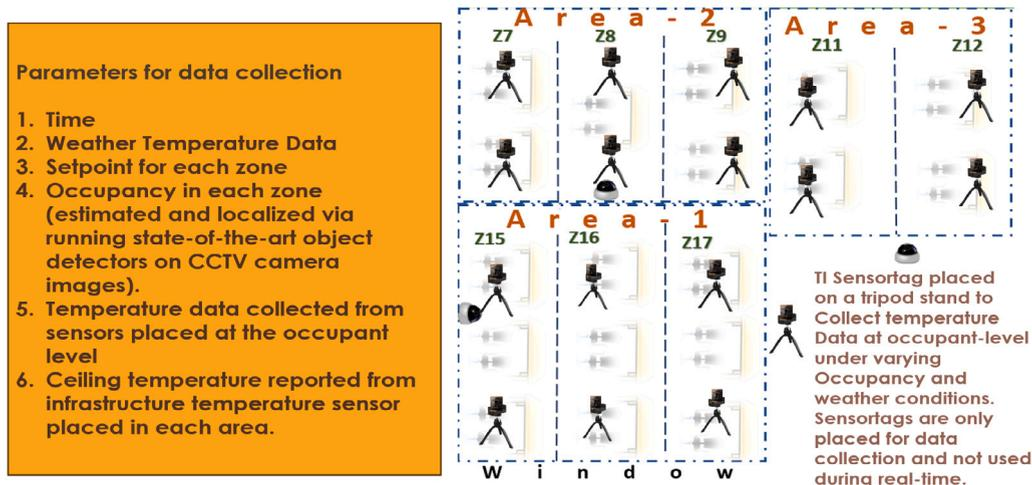
Fig. 3. Data collection setup and parameters collected.
