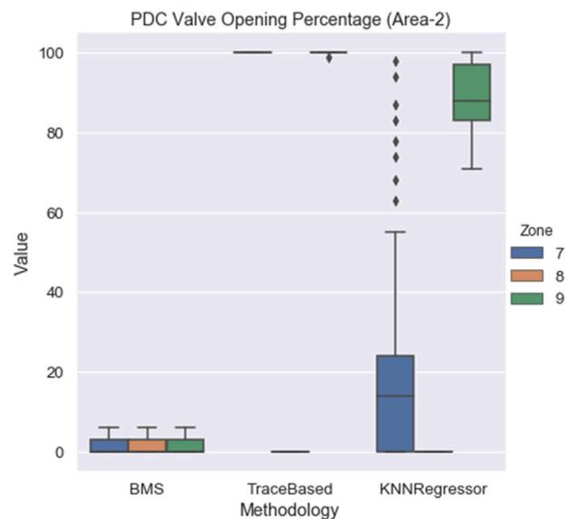
Fig. 20. PDC valve opening percentage for BMS Vs OcAPO (TraceBased and KNN regressor) across all 3 zones (Area-2).
