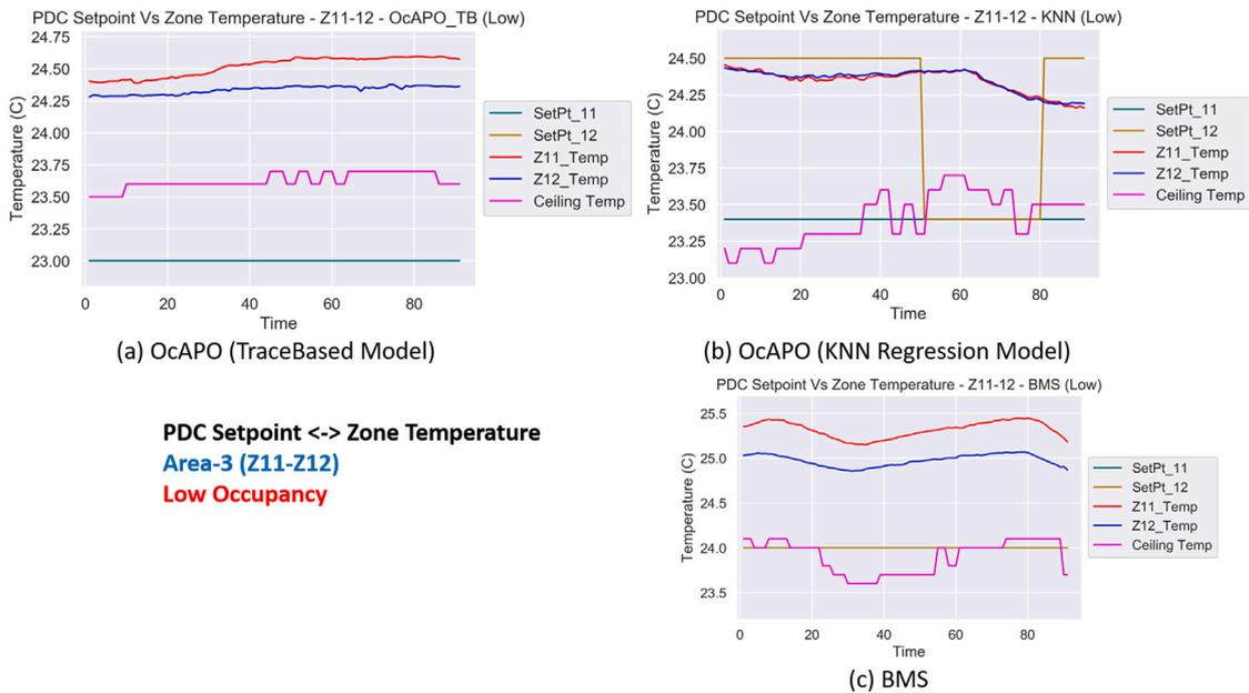
Fig. 14. PDC setPoint by BMS, OcAPO (TraceBased and KNN) Vs ceiling and zone temperature — low occupancy (Area-3).
