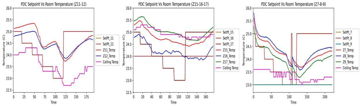
Fig. 8. Recorded room temperature for varying PDC setpoints.
