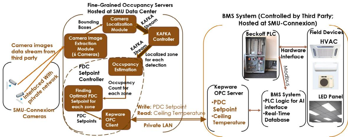
Fig. 12. Modules in OcAPO and interaction with BMS (Building Management System).
