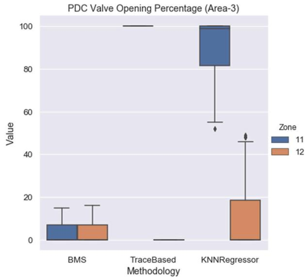
Fig. 19. PDC valve opening percentage for BMS Vs OcAPO (TraceBased and KNN regressor) across all 3 zones (Area-3).
