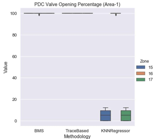
Fig. 21. PDC valve opening percentage for BMS Vs OcAPO (TraceBased and KNN regressor) across all 3 zones (Area-1).
