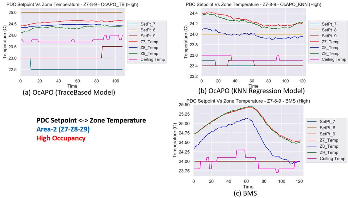
Fig. 15. PDC setPoint by BMS, OcAPO (TraceBased and KNN) Vs ceiling and zone temperature — high occupancy (Area-2).
