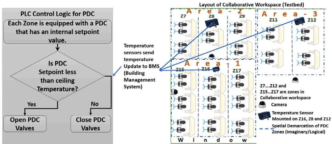
Fig. 2. Layout of collaborative workspace (Testbed) and interface with BMS.
