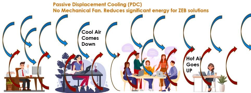
Fig. 1. Working principle of Passive Displacement Cooling (PDC).
