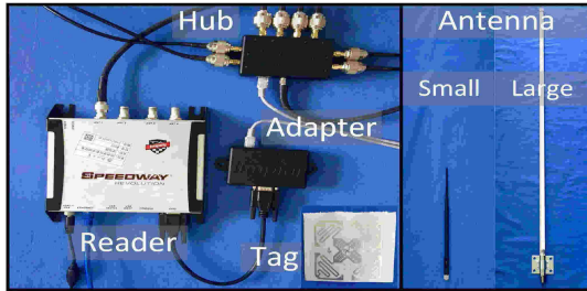
Fig. 9. RFID hardware and antennas employed.
