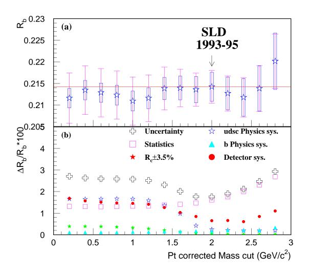
Figure 3: (a) Variation of  $R_b$  with the  $\mathcal{M}$  cut. The statistical error is represented by the boxes and the outer bars show the sum in quadrature of the statistical and systematic errors. (b)  $R_b$  statistical and systematic uncertainties versus  $\mathcal{M}$  cut.
