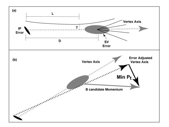
Figure 1: (a) An illustration of the SV track attachment criteria. (b) Illustration of the  ${\cal P}_t$  derivation.
