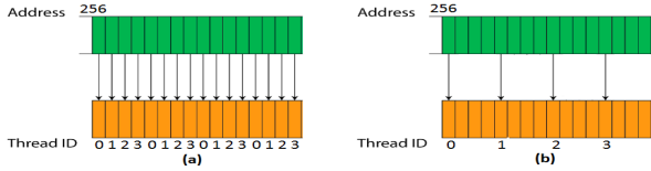
Figure 5: Memory Coalescing vs Memory Vectorization
