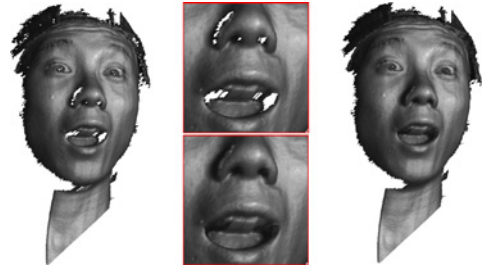
Fig. 3. Captured raw data usually contains holes due to the occlusions. We fill both the geometry and texture of the holes by constructing a minimal surface which has C^1 continuity along the hole boundaries.
