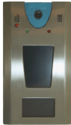
Figure 5: An XID Access control Device developed for in – situ building installation
